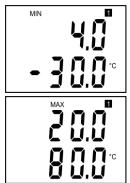
Range and type of value for output 1 (current loop II = symbol ",1" on display). Type of value, assigned to output 1, is indicated by displayed unit (here °C). Upper line displays current value corresponding to measured value (lower line). Here 4 mA corresponds to -30 °C.
