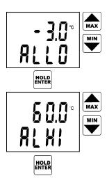
It is possible to set lower and upper limit for measured temperature. Breaking of the limit is indicated by blinking of the value on the display. Alarm activation can be disabled by setting lower alarm limit up to its maximum. This is indicated by OFF reading at the position of numeric value. Value of upper limit of the same alarm is indifferent.
